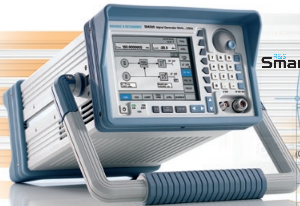
FIG 1 The Vector Signal Generator R&S® SM300, the new member of the R&S Smart Instruments™ family.
