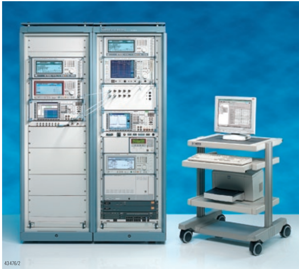
FIG 1 Test System R&S® TS 8950 GW for conformance tests of GSM/WCDMA mobile phones. The test system's ability to perform such high-precision measurements is the result of sophisticated calibration methods and software specially developed by Rohde & Schwarz.
