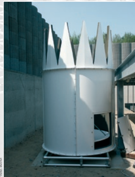
Powerful loudspeaker towers expand the radar system to form a RASS for measuring virtual temperature. They generate a sound pressure of 135 dBa at a height of 2 m.
